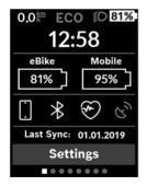
As well as the status bar, the status page also shows you the current time and the state of charge of all your eBike's batteries, as well as the state of charge of your smartphone battery if the smartphone is connected via Bluetooth®.
